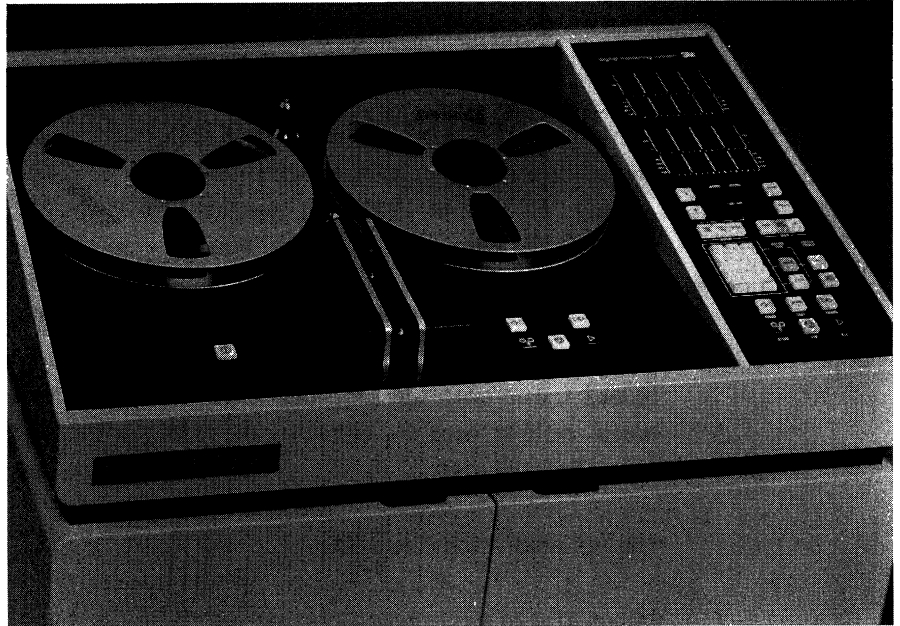
Figure 1.6 3M 32-track digital tape recorder, introduced in 1978.
