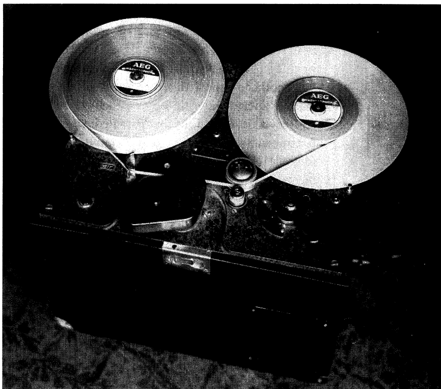
Figure 1.3 Prototype of a portable Magnetophon tape recorder from 1935, made by AEG. (Photograph courtesy of BASF Aktiengesellschaft.)
