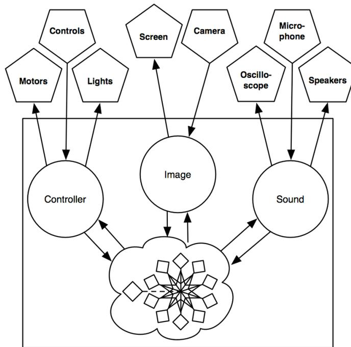
**Figure 33. Software Architecture of *DEFENDEX-ESPGX*.**
