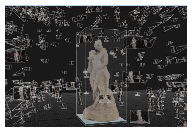
Photogrammetry is a 3D recording technique that employs 2D images to create a 3D model of an object or surface. It involves taking hundreds of overlapping photographs of an object from many different angles and processing them using specialised software such as <a href="RealityCapture">RealityCapture</a> (RC) or Agisoft PhotoScan. The digital 3D model can be used for study or outputted as a physical object via 3D printing or CNC milling.
