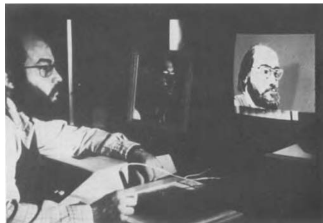
Fig. 13. Duane Palyka, Painting Self-Portrait , 1975. (Photo: Mike Milocheck). The artist painted a self-portrait on a computer at the University of Utah Computer Science Department in 1975. In the picture, Palyka is using a simple paint program called Crayon, written in Fortran by Jim Blinn. The program ran under the DOS operating system on a DEC PDP-11/45 using the first Evans & Sutherland frame buffer.
